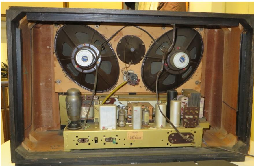
bottom side of this electronic device chassis, accessible from the bottom of the wooden radio mainframe, are the very electronic components, like the smaller resistors, capacitors and inductors. They are mounted towards the bottom to prevent from accumulating dust, what would have affected the electronic performance, and -not to forget- could also lead to inflammation due to the heated tubes.
