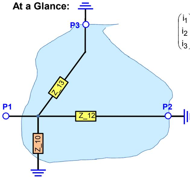
$$\begin{pmatrix} i_1 \\ i_2 \\ i_3 \end{pmatrix} = \begin{pmatrix} Y_{11} & Y_{12} & Y_{13} \\ Y_{21} & Y_{22} & Y_{23} \\ Y_{31} & Y_{32} & Y_{33} \end{pmatrix} \cdot \begin{pmatrix} v_1 \\ v_2 \\ v_3 \end{pmatrix}$$
