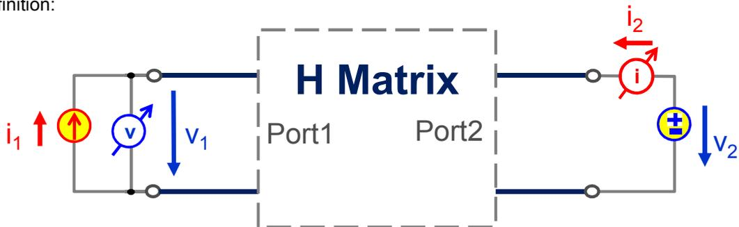
$$\begin{matrix} \text{measured} \\ \begin{pmatrix} v_1 \\ i_2 \end{pmatrix} \end{matrix} = \begin{pmatrix} H_{11} & H_{12} \\ H_{21} & H_{22} \end{pmatrix} * \begin{matrix} \text{stimulated} \\ \begin{pmatrix} i_1 \\ v_2 \end{pmatrix} \end{matrix}$$
