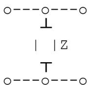
and the Z-matrix is not defined for a series-impedance-only Two-Port like this:
