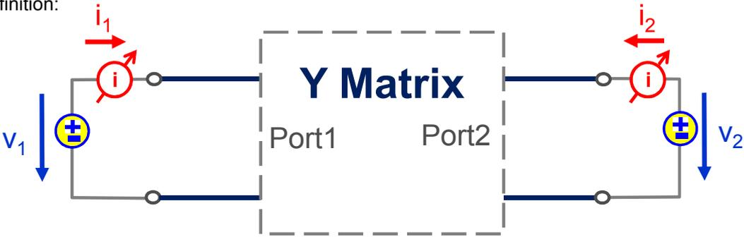
The diagram shows a two-port network enclosed in a dashed box labeled "Y Matrix". The left port is labeled "Port1" and the right port is labeled "Port2". At Port1, a voltage source  $V_1$  is connected in series with the port, and the current  $i_1$  is measured entering the port. At Port2, a voltage source  $V_2$  is connected in series with the port, and the current  $i_2$  is measured entering the port.
