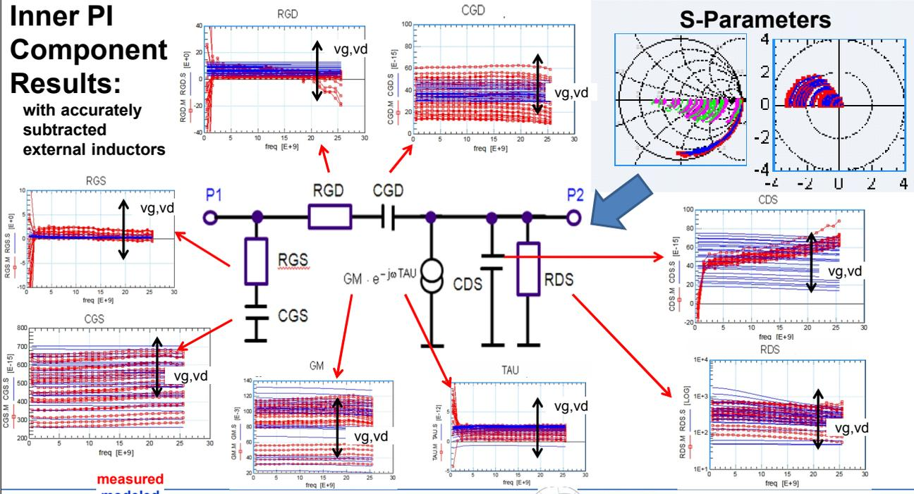
A typical measurement verification result, with correctly stripped-off external inductors: only very little dependency of the Inner-PI-schematic components versus frequency.
