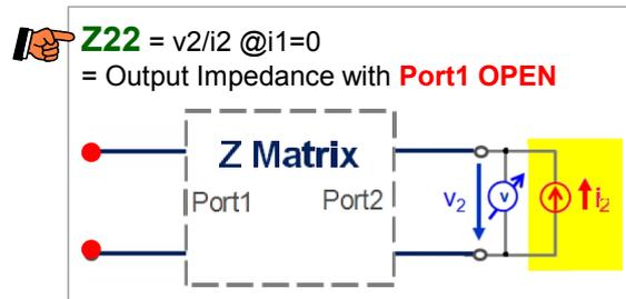
**Application: Verification of Passive Components Modeling**
