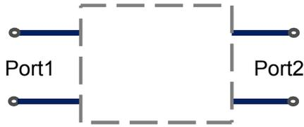
$$\begin{pmatrix} v_1 \\ v_2 \end{pmatrix} = \begin{pmatrix} Z_{11} & Z_{12} \\ Z_{21} & Z_{22} \end{pmatrix} * \begin{pmatrix} i_1 \\ i_2 \end{pmatrix}$$
