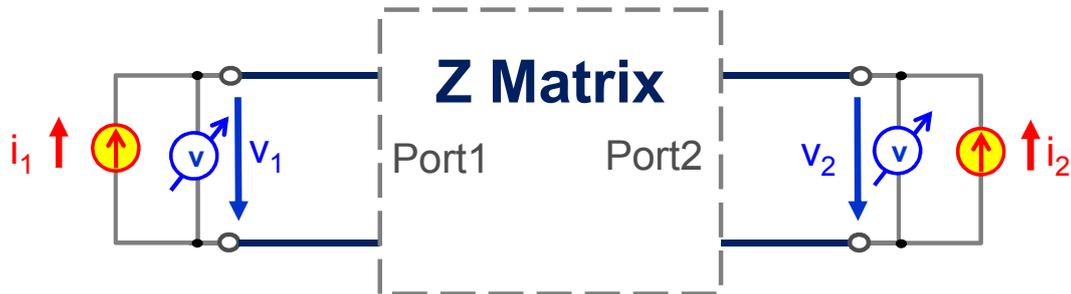
$$\begin{matrix} \text{measured} \\ \begin{pmatrix} v_1 \\ v_2 \end{pmatrix} \end{matrix} = \begin{pmatrix} Z_{11} & Z_{12} \\ Z_{21} & Z_{22} \end{pmatrix} * \begin{matrix} \text{stimulated} \\ \begin{pmatrix} i_1 \\ i_2 \end{pmatrix} \end{matrix}$$
