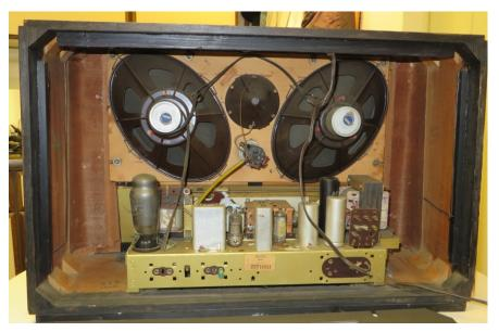
bottom side of this electronic device chassis, accessible from the bottom of the wooden radio mainframe, are the very electronic components, like the smaller resistors, capacitors and inductors. They are mounted towards the bottom to prevent from accumulating dust, what would have affected the electronic performance, and -not to forget- could also lead to inflammation due to the heated tubes.
