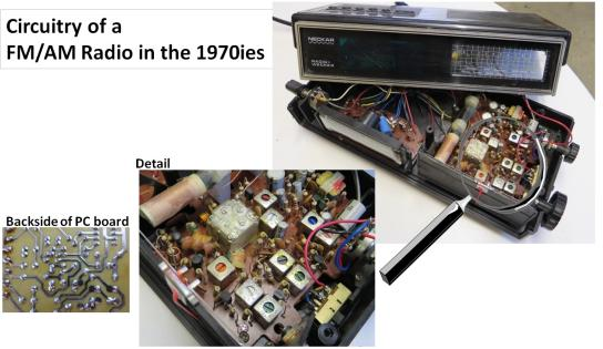
The circuit board, made from epoxy, holds on one side the components, while the back side is used for connecting the components with cupper areas etched out of the copper foil PCB layer. The circuitry therefore is now much more compact and the component placing and later soldering can already be done by automates.
