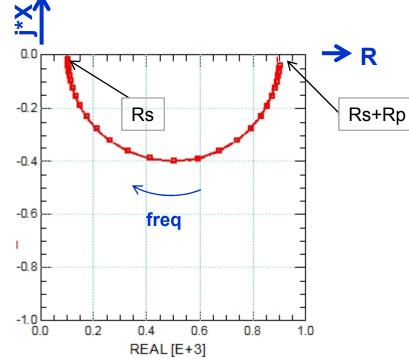
Impedance Plot Explanations: freq -> 0: Cp is an OPEN: Z=Rp+Rs is at the right x-axis freq -> infinite: Cp shorts Rp: Z=Rs
