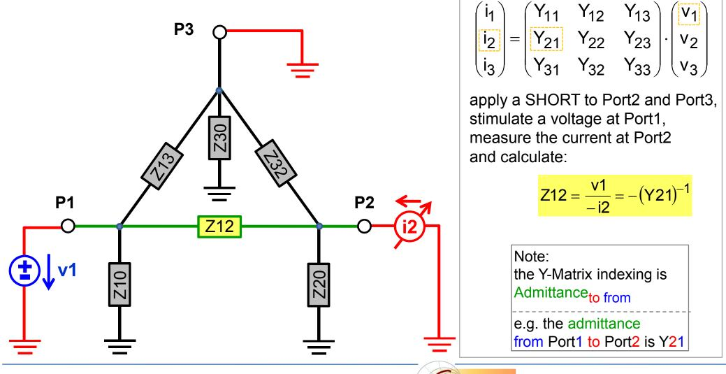
Note: for the Y-matrix, mind the currents into the DUT
