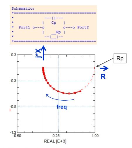
Impedance Plot Explanations: freq -> 0: Cp is an OPEN, Z=Rp freq -> infinite: Cp shorts Rp (Z=0) in between: a half-circle turning from Rp clock-wise (with increasing freq) to Z=0
