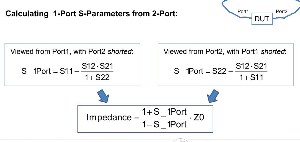
Impedance Plots can also be obtained from S-Parameter Measurements
