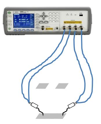
The impedances of two Calibration Standards are measured first
