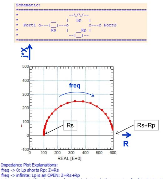
in between: a half-circle turning from Rs clock-wise (with increasing freq) to Z=Rs+Rp
