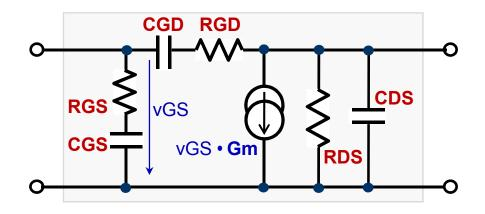
1. Convert de-embedded S-parameters to Z, and strip-off external inductors and resistors
