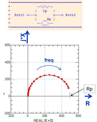
Impedance Plot Explanations: freq -> 0: Lp is a SHORT: Z=0 freq -> infinite: Lp is an OPEN, Z=Rp in between: a half-circle turning from Z=0 clock-wise (with increasing freq) to Z=Rp
