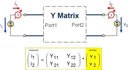
The Y-matrix is very useful when the impedances between the ports need to be extracted and analyzed, especially for multi-port applications. This is due to the voltage stimulation at the ports.
