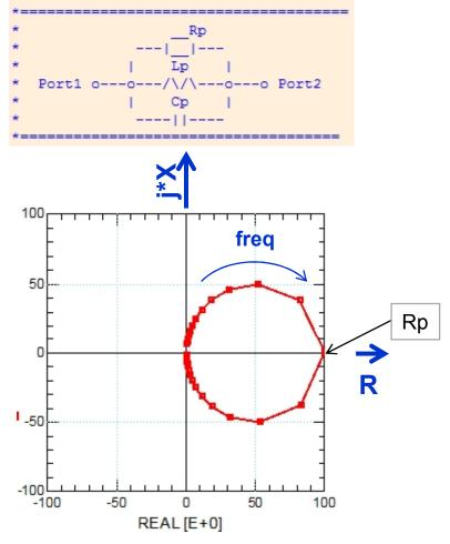
Impedance Plot Explanations: freq -> 0: Lp is a SHORT, Z=0 resonance: the x-axis is crossed at Rp freq -> infinite: Cp is a SHORT, Z=Rp
