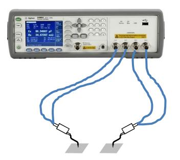
The impedances of two Calibration Standards are measured first
