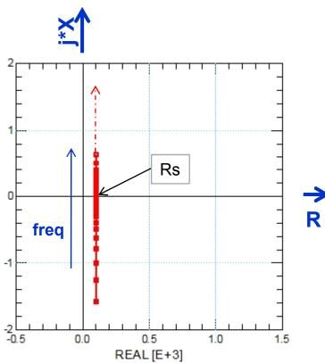
Impedance Plot Explanations: freq -> 0: Cs is an OPEN: Z=-j\*infinite freq -> infinite: Ls is an OPEN: Z=j\*infinite — in between: resonance: Z=Rs with increasing freq, a straight line bottom -> up from Z=-j\*infinite, towards Z=Rs (resonance), and the further up to Z=j\*infinite
